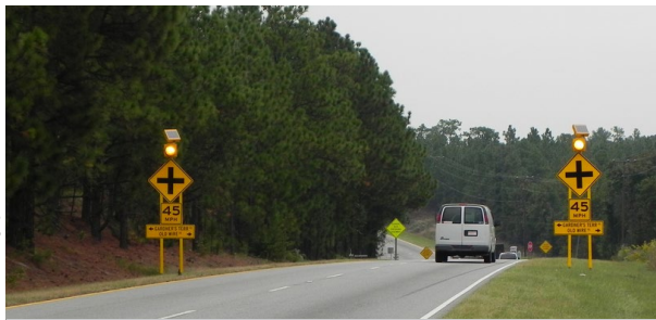
Example of countermeasures on the through approach.
