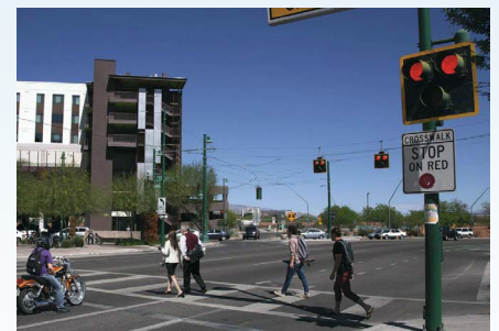
Pedestrians cross the roadway at a PHB location.
