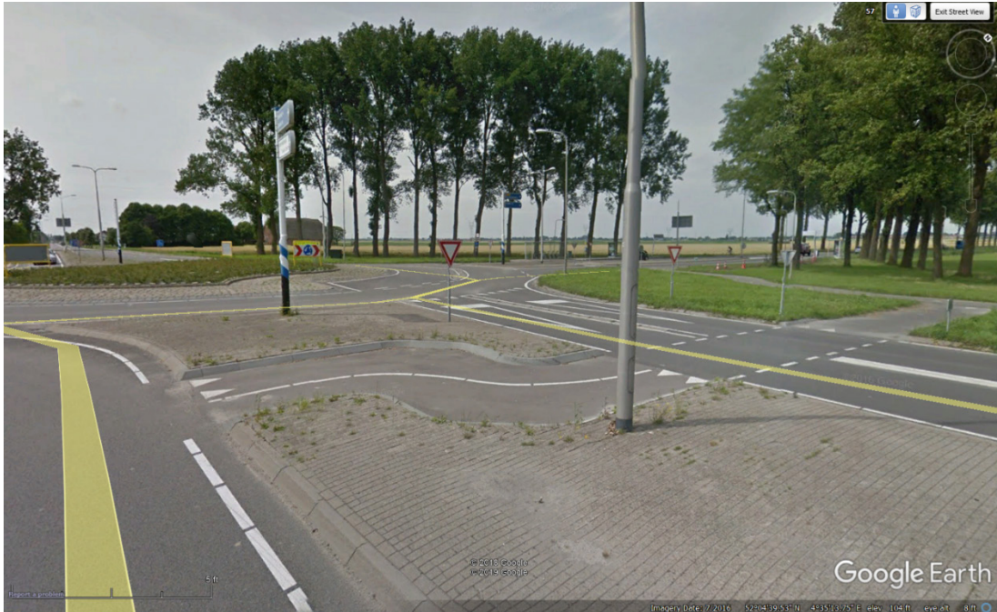
Figure 17. Photograph. Example of a chicane in a splitter island at a turbo roundabout in the Netherlands to provide additional time for approaching drivers to identify the bicyclist and to encourage bicyclists to perform a two-stage crossing. (32)
