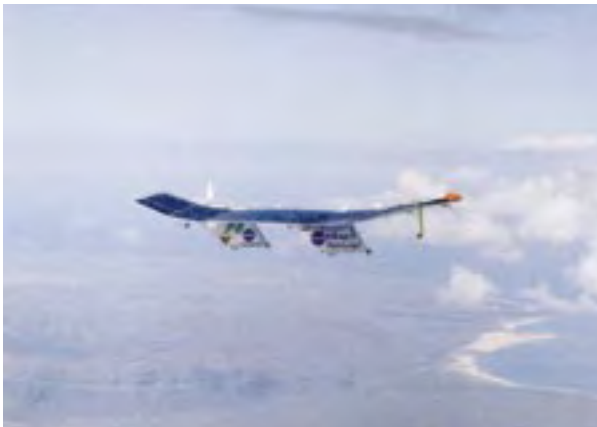
Unmanned solar plane powered by a renewable regenerative fuel cell (Courtesy: Aerovironment)
