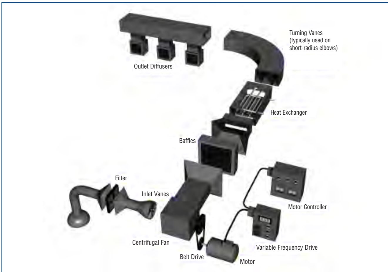
Figure 1-3. Example Fan System Components
