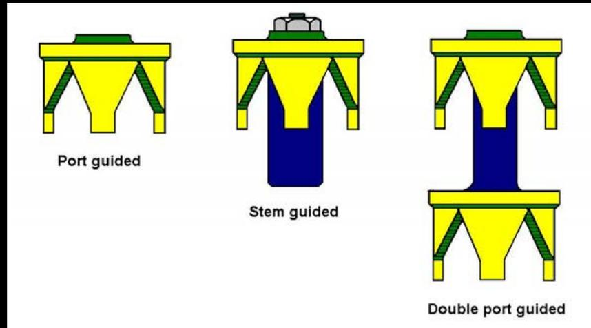
Figure 27 - Modified parabolic or "vee" plugs
