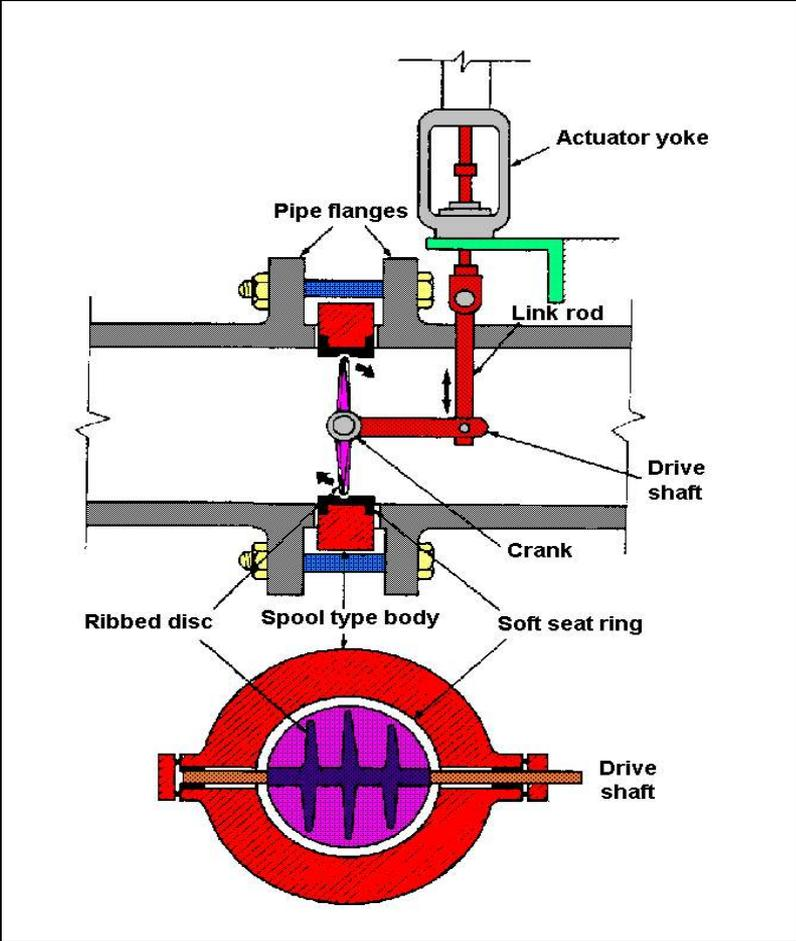
Figure 17 - Butterfly valve in flangeless spool
