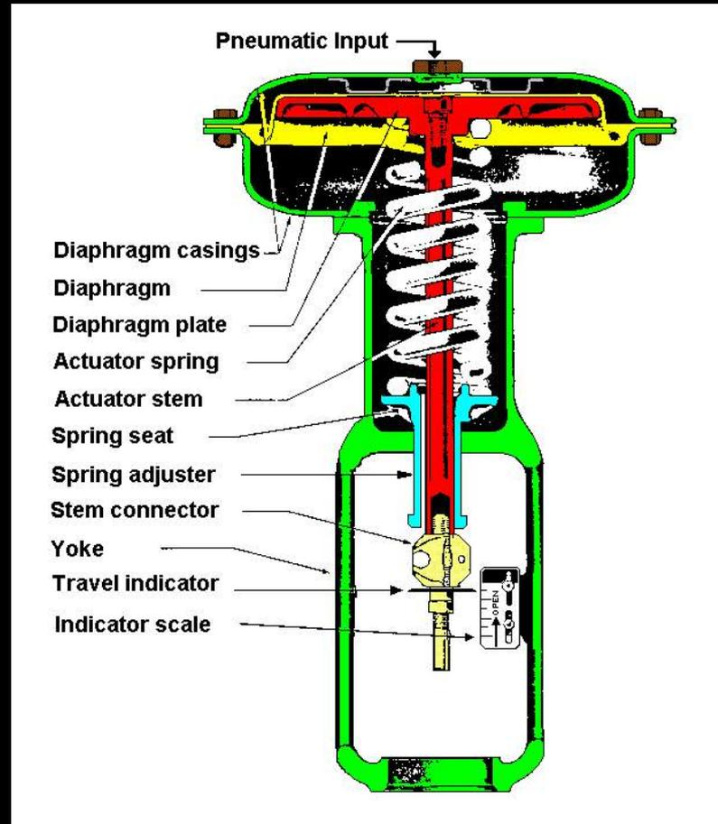
Figure 29 - Direct acting actuator
