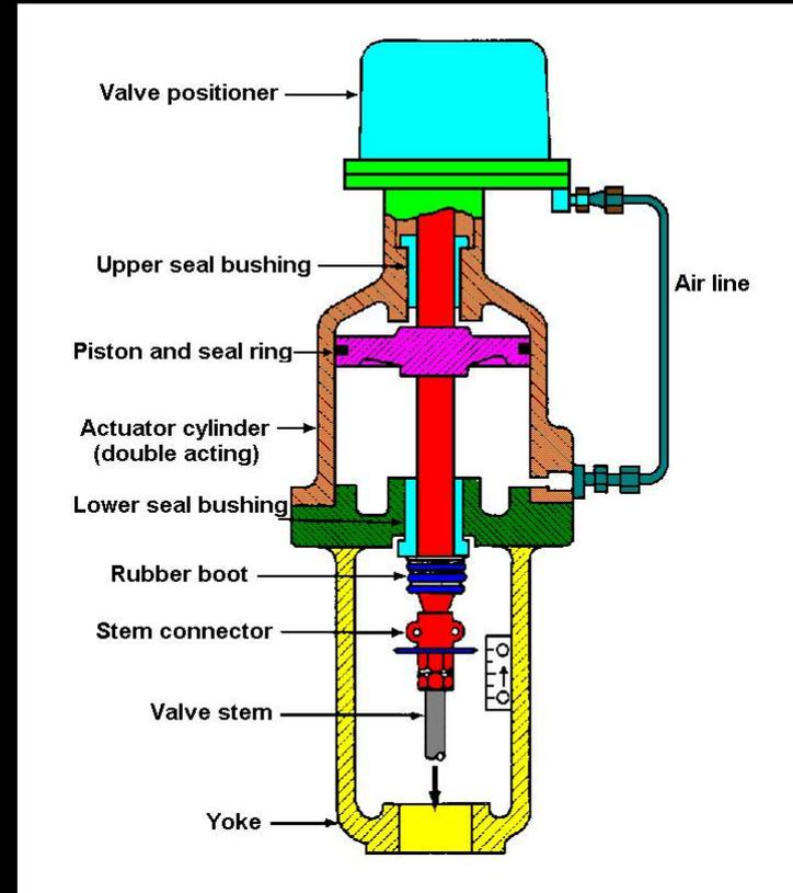
Figure 31 - Pneumatic piston actuator
