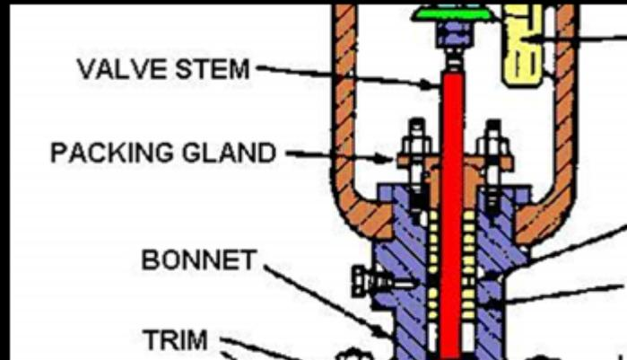
Figure 4 - Typical packing box assembly
