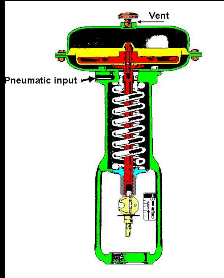
Figure 30 - Reverse acting actuator
