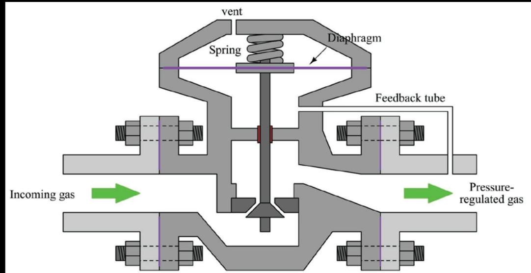
Figure 35 – Feedback self-operated control valve
