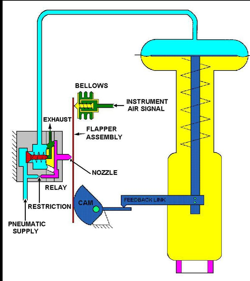
Figure 37 - Pneumatic valve positioner (simplified)
