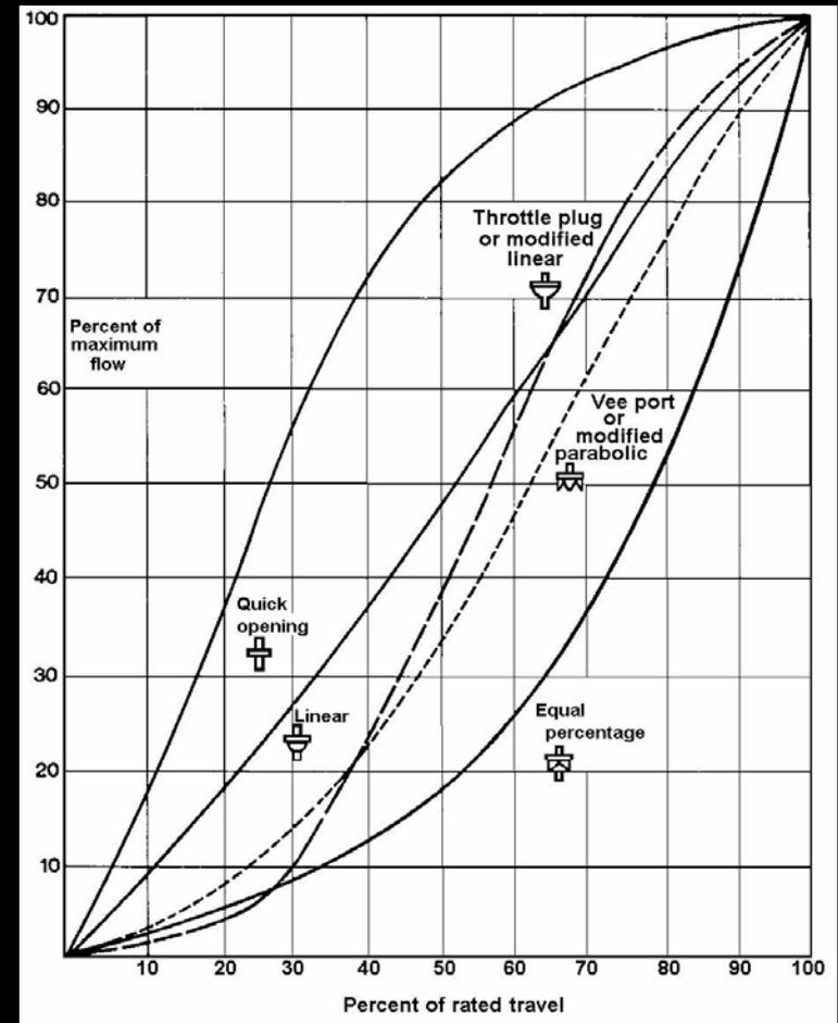
Figure 22 - Flow characteristics for control valves
