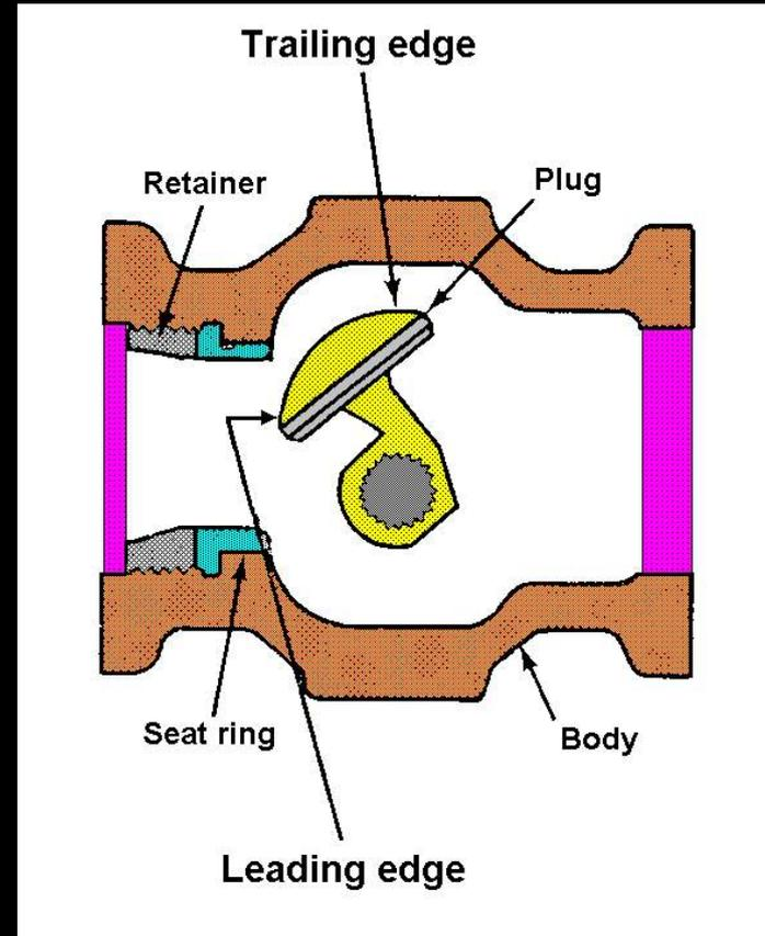
Figure 20 - Rotary eccentric plug valve
