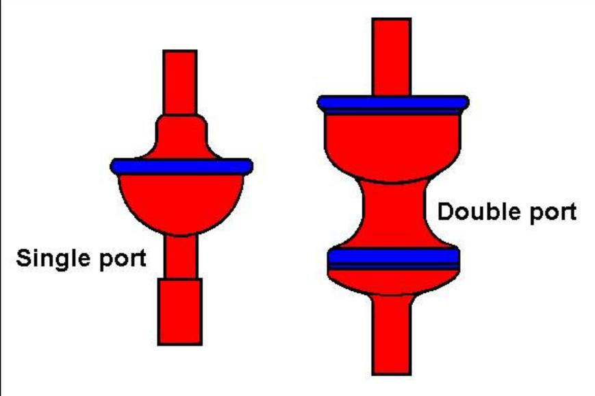
Figure 25 - Modified linear or throttle plugs
