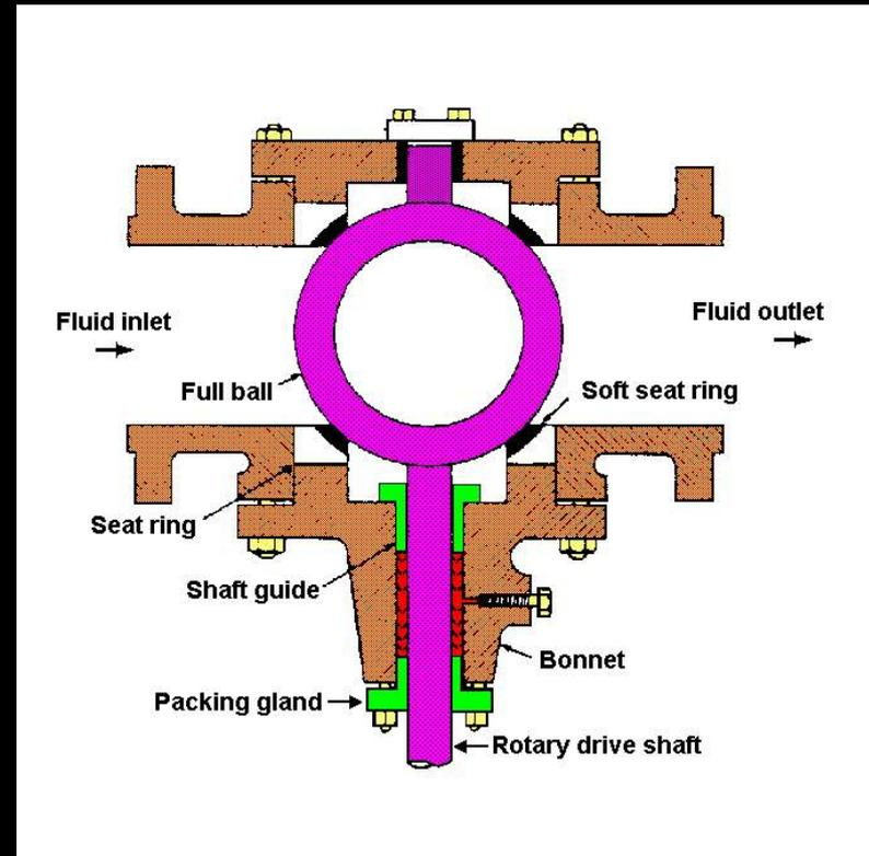
Figure 19 - Ball valve - plan view
