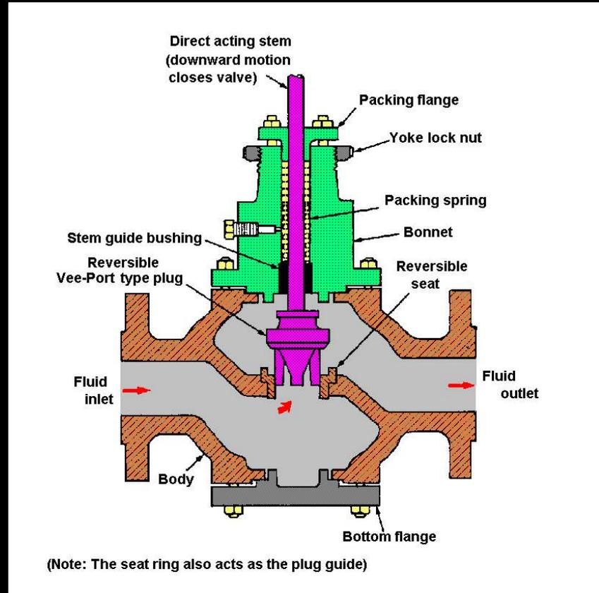
Figure 13 - Single port unbalanced reversible plug valve
