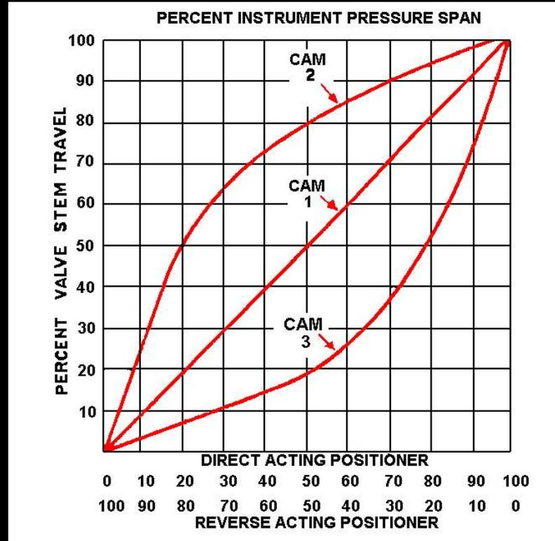
Figure 38 – Typical cam characteristics
