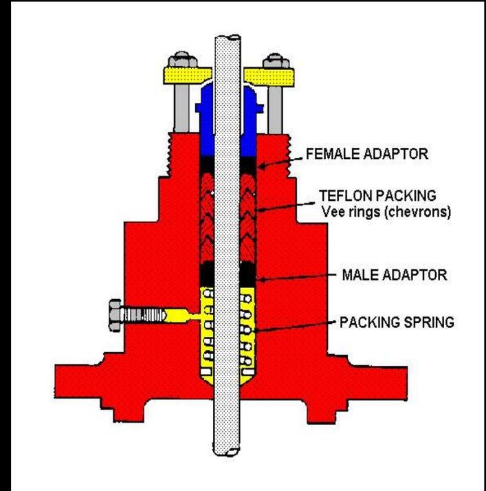
Figure 6 - Typical non lubricated packing box
