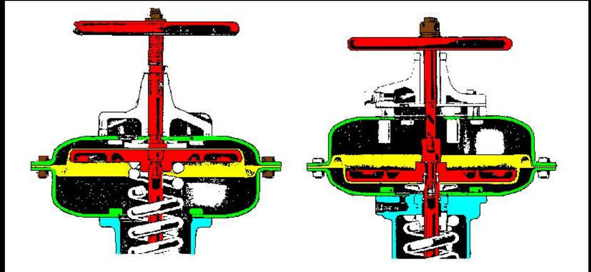
Figure 32 - Top mounted hand-wheels
