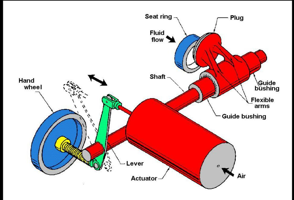
Figure 21 - Rotary eccentric plug valve and actuator
