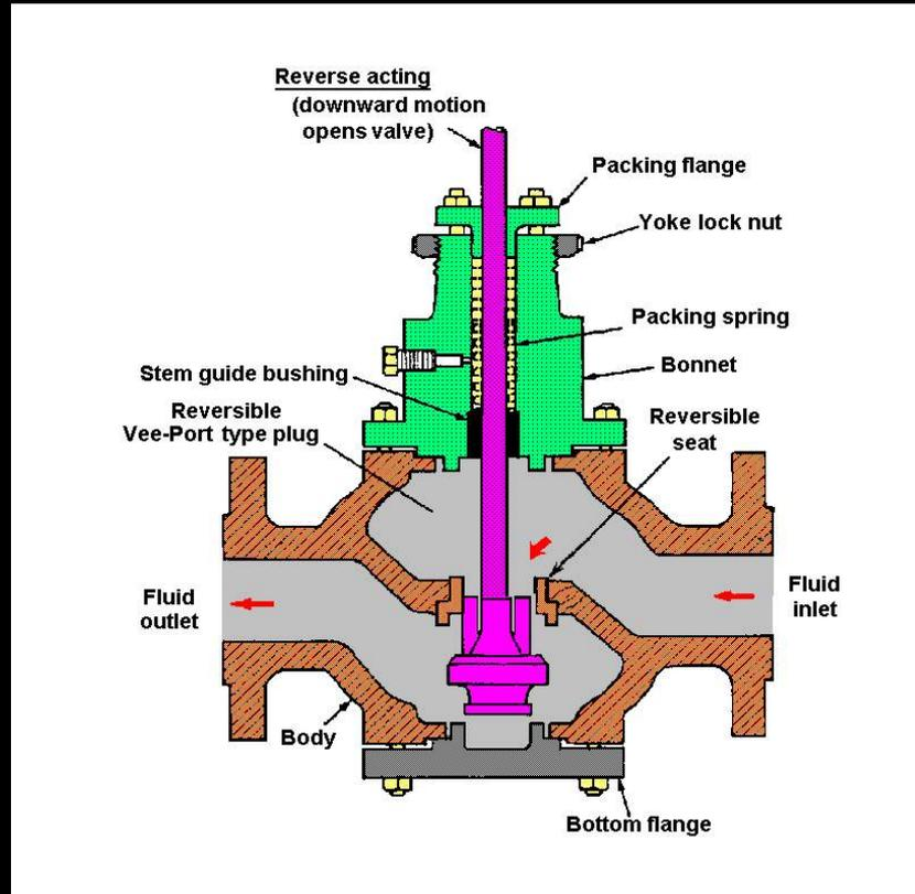
Figure 14 - Single port valve with plug reversed
