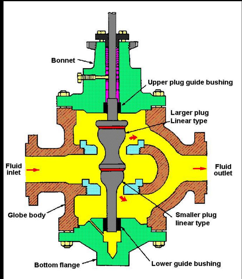
Figure 15 - Double port semi-balanced valve
