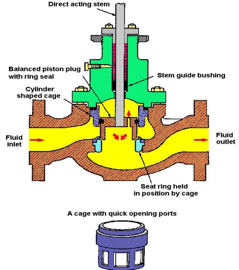
Figure 16 - Single port cage-trim piston valve
