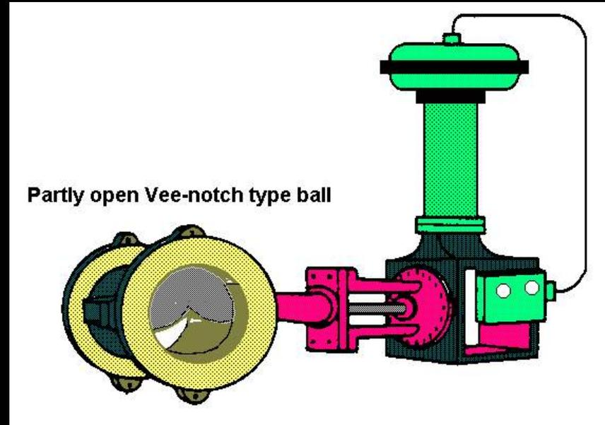
Figure 18 - Ball valve and diaphragm actuator assembly
