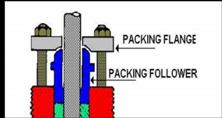
Figure 7 - Typical packing flange
