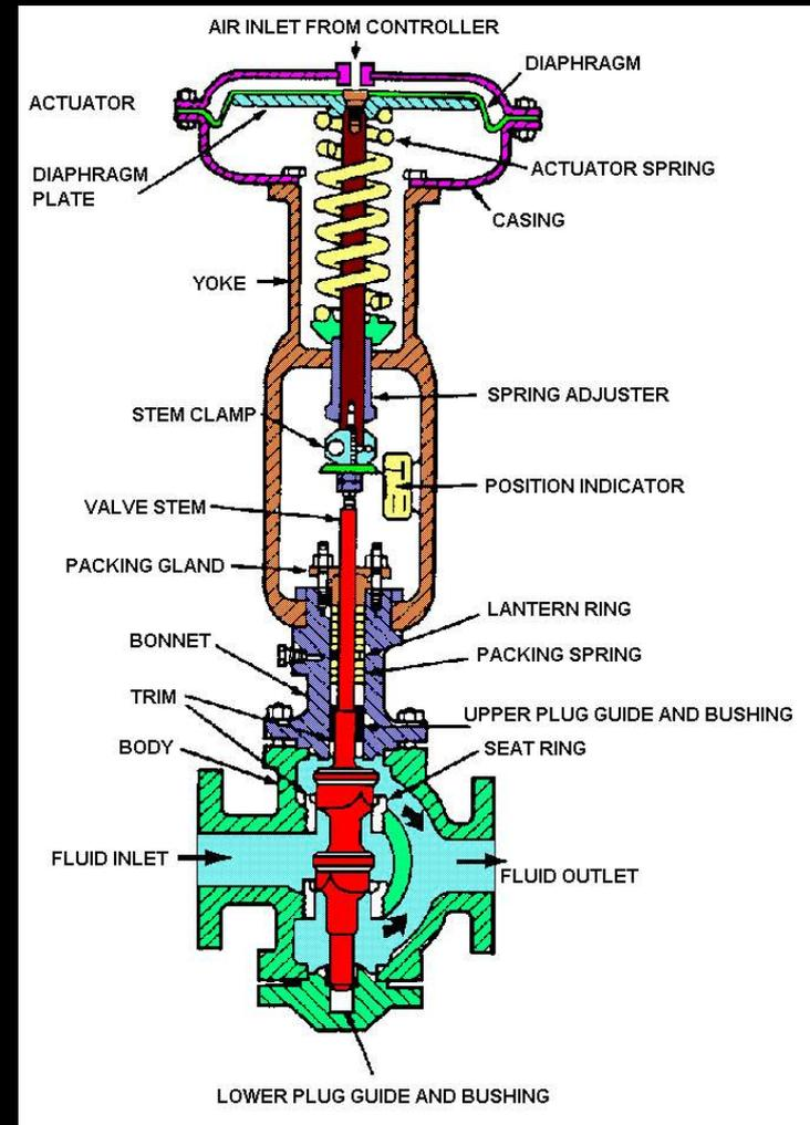
Figure 1- Typical control valve
