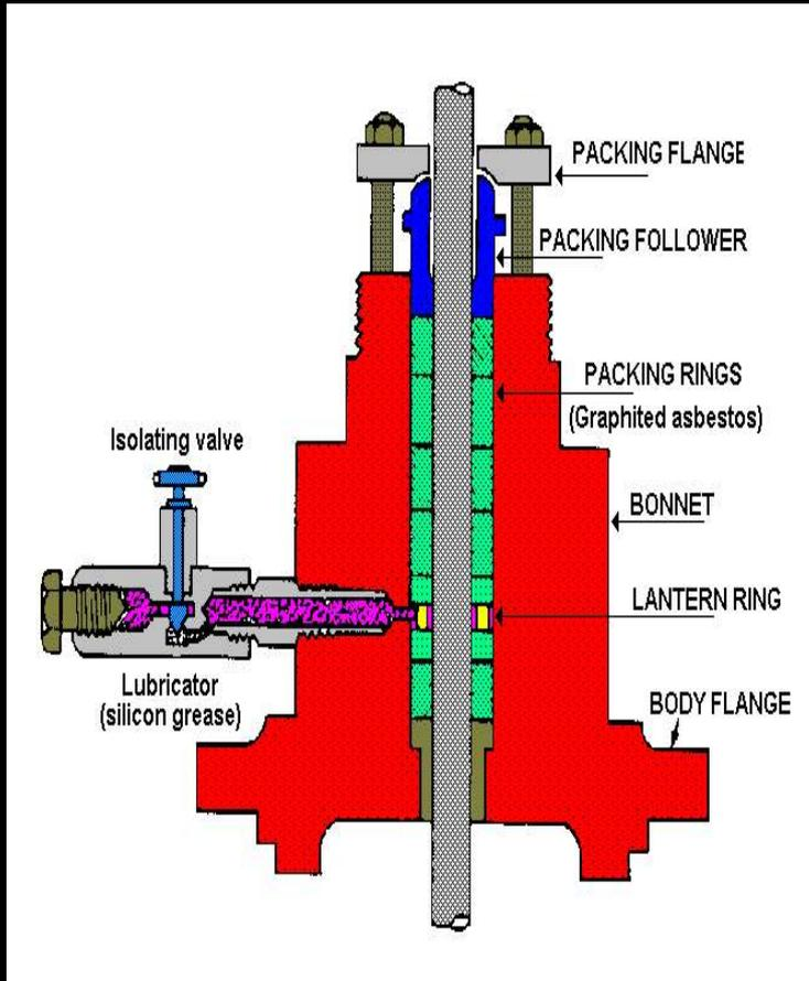
Figure 5 - Typical packing box
