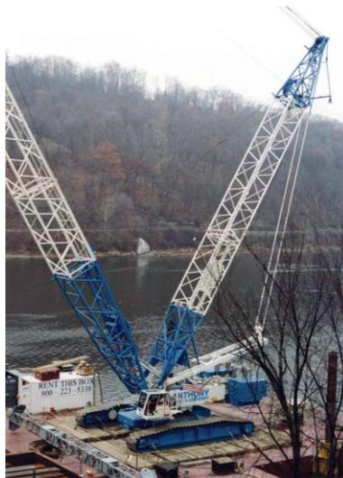
**Figure 3 Photograph of a lattice boom crawler crane**
