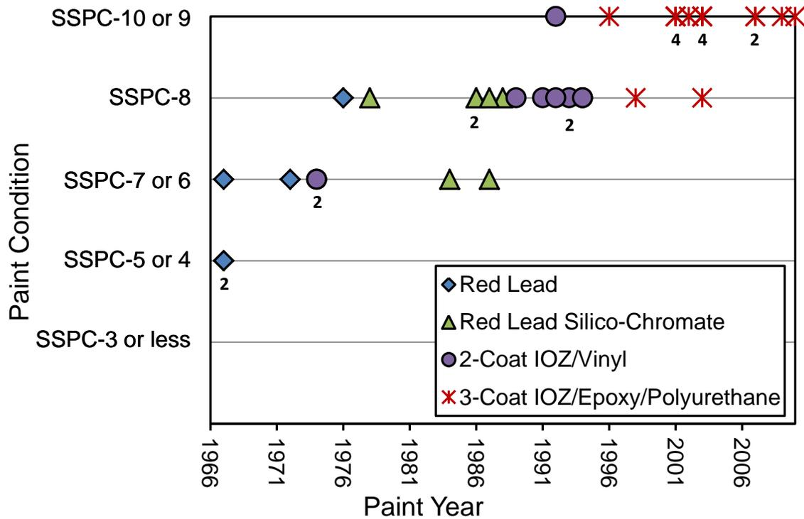
Figure 12. Graph. Condition ratings of original coating systems in Missouri (numbers by data points represent replicates).<sup>(reproduced from 61)</sup>
