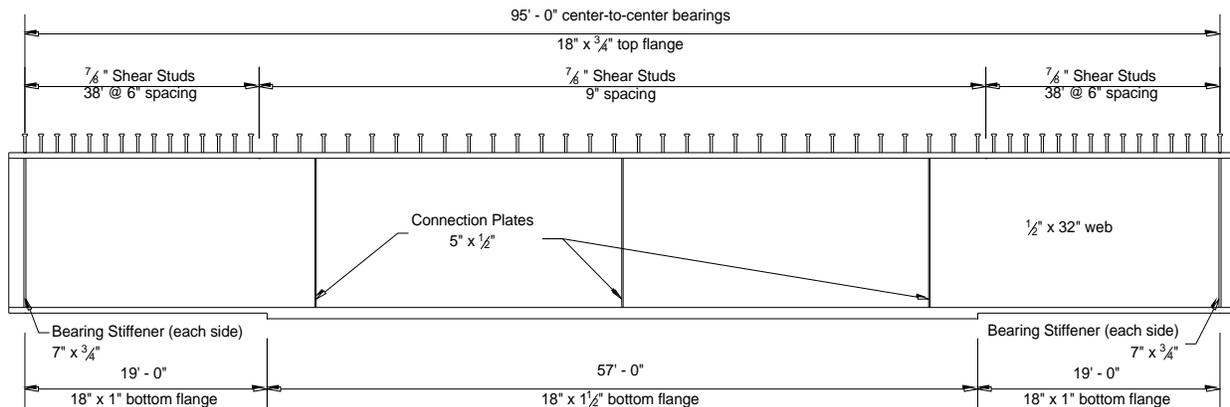
Figure 42. Schematic. Elevation view of girder detailing.
