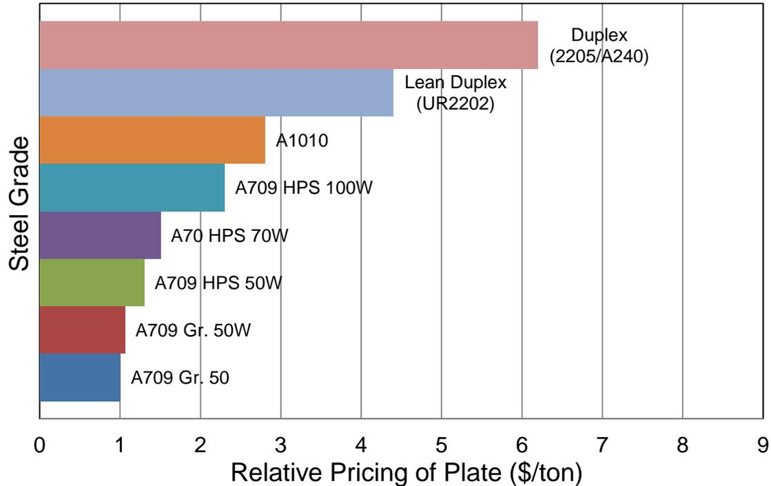
Figure 41. Graph. Relative pricing of various steel alloys.
