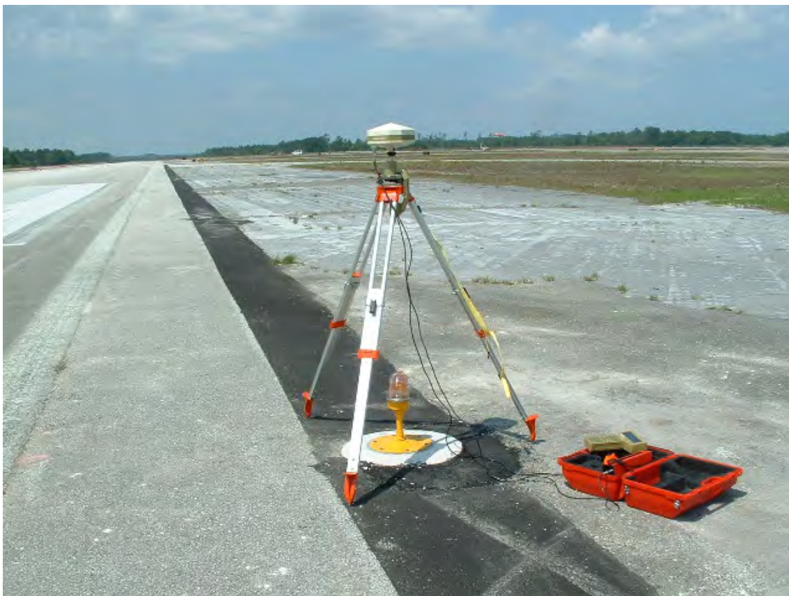
Figure 2-3. Airfield NAVAID positioning using Fast-Static GPS methods
