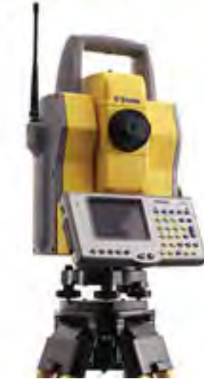
Figure 8-6. Trimble 5600 DR Reflectorless-Robotic Total Station with ACU Survey Controller
