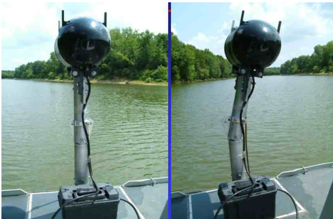
Figure 6-12. Bow-mounted transducer with an optional rigid (locking) tilt capability to provide coverage up to water's edge on revetments or lock & dam structures. This rigid tilt lock minimizes the need for Patch Testing at this optional setting. (St. Louis District S/V Boyer)
