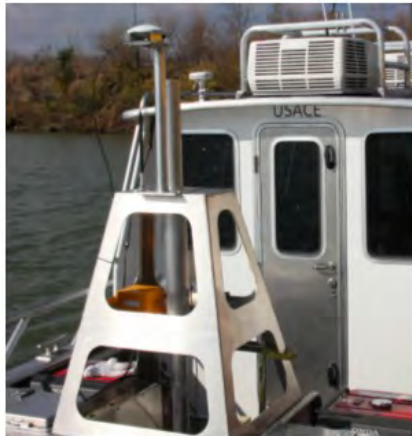
Figure 6-8. Louisville District 30-ft survey boat with through hull mounted transducer (Reson 8125-H multibeam system).
