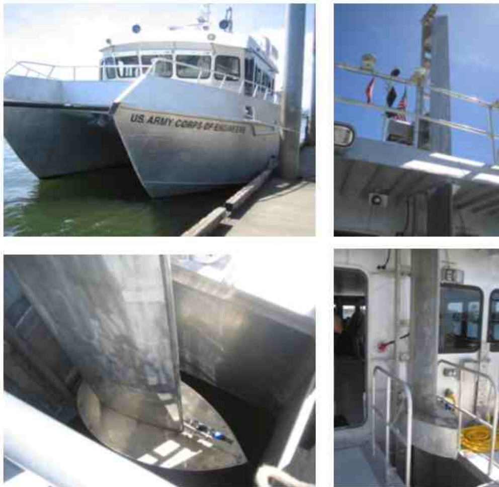
Figure 6-7. Portland District S/V Redlinger. The S/V Redlinger is a 60-ft foil supported catamaran. Survey equipment includes an Applanix POS/MV, Simrad EM 3002, and an Odom CV100. The transducer is located just aft of the cabin.
