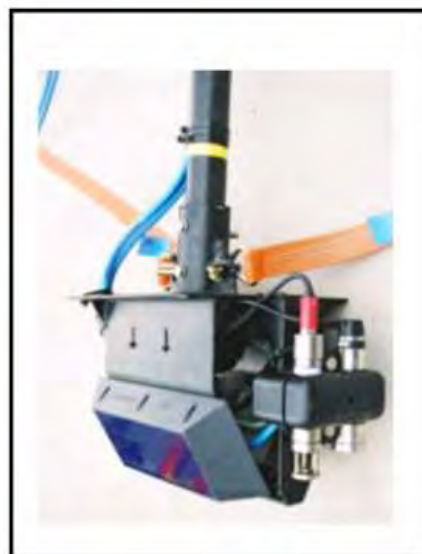
Figure 6-13. Typical multibeam transducer systems side-mounted on a rigid pole attached to the survey vessel. (Odom, Inc. and GeoAcoustics, Inc.)
