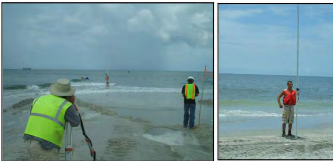
Figure 11-4. Beach profiles using a level and tagline for control. On left photo, fixed end of tag line is held at TBM next to grade stake. Range poles or grade stakes are used for visual alignment. Rodman on right photo is shown with 25-ft level rod.
