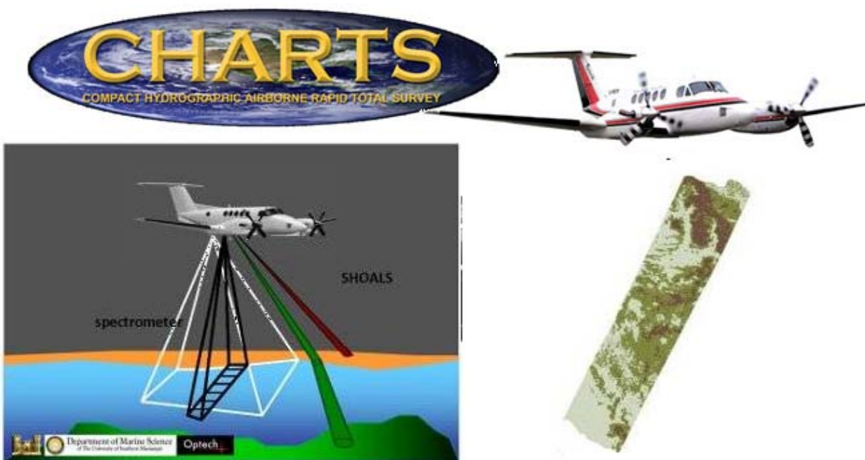
Figure 6-14. USACE GPS-controlled CHARTS hydrographic surveying system (JALBTCX)
