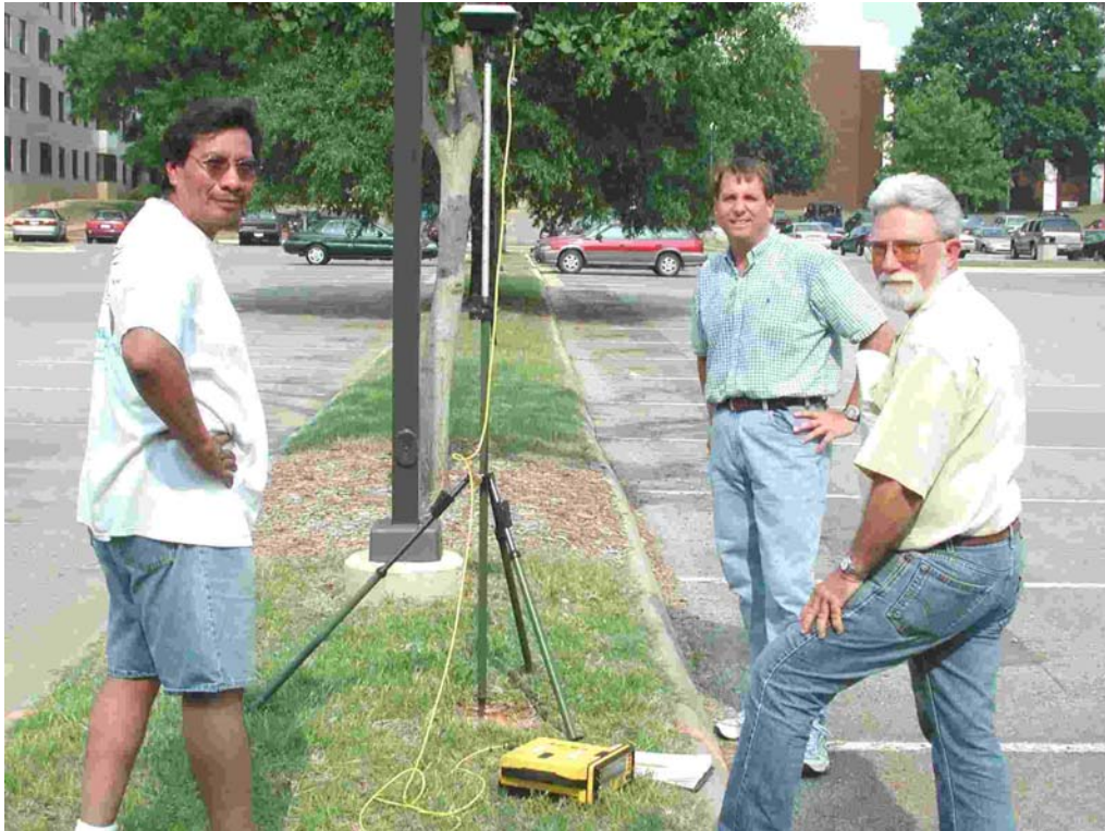
Figure 6-2. Fast-Static control survey of topographic reference monument at Huntsville Beville Center
