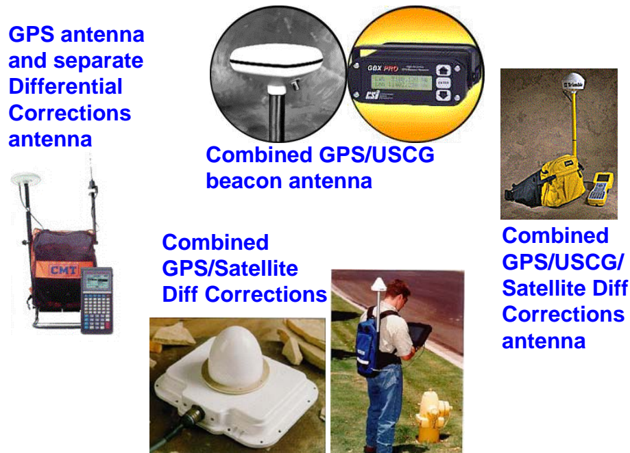
Figure 7-3. Common data links for code and RTK GPS receivers
