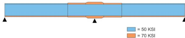
**Figure 9 Diagram of a hybrid steel I-girder**
