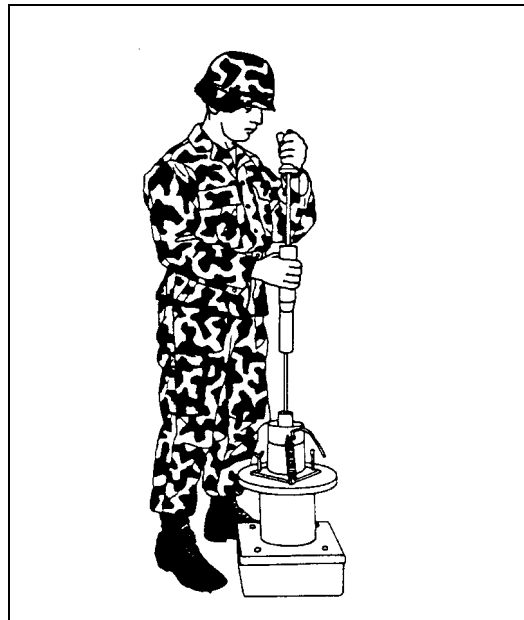
Figure 3-14. Compaction of bituminous trial-mix specimens
