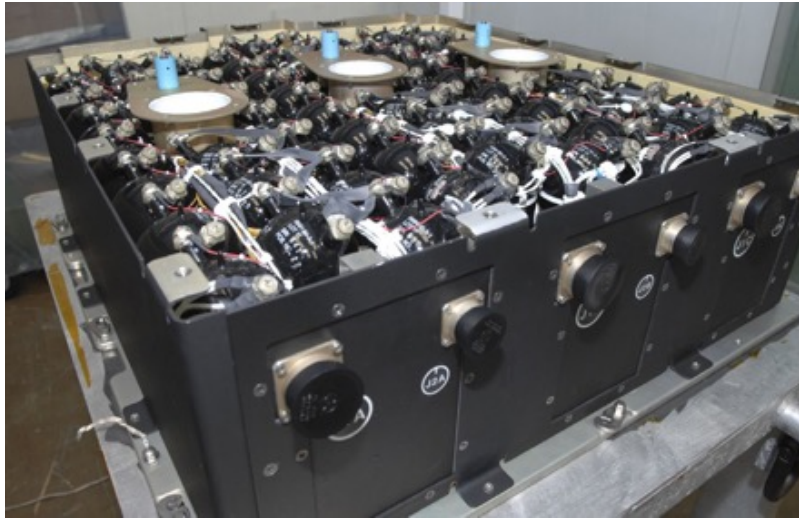
The Hubble space telescope's nickel-hydrogen battery module (NASA)
