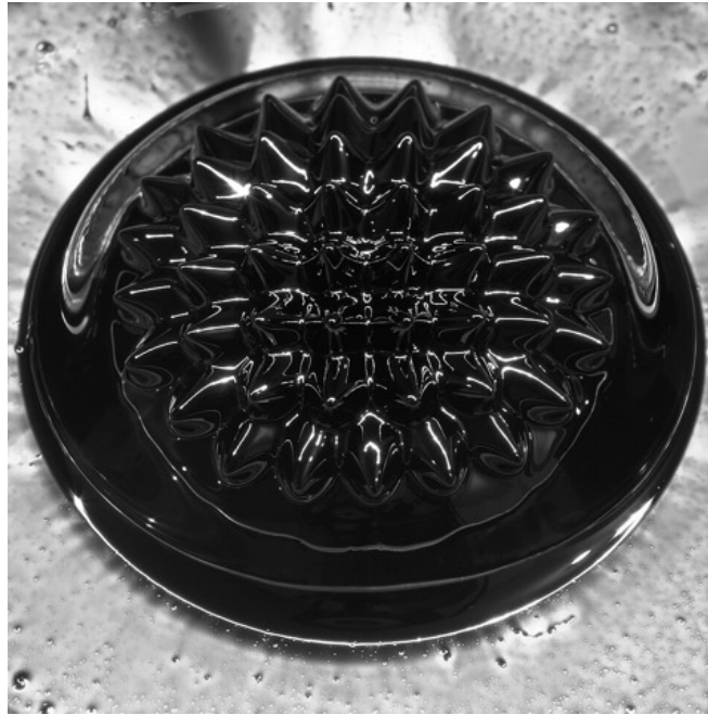
Figure 5: Spike Pattern in Ferrofluid Under Magnetic Field
