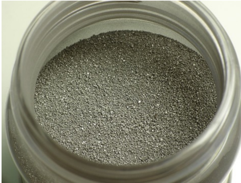
Figure 2: Magnetizable fine iron powder
