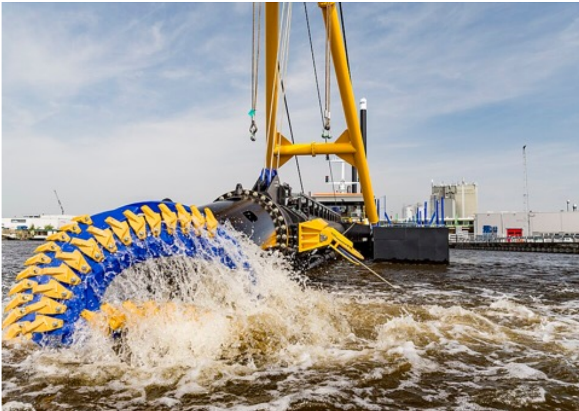
Figure 4: Cutter Suction Dredgers (CSDs)
