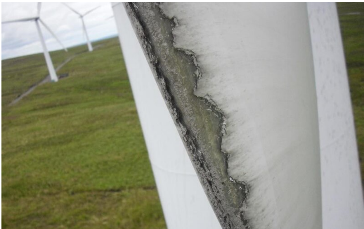
Figure 2: Water droplet erosion damage in wind turbines caused by rain
