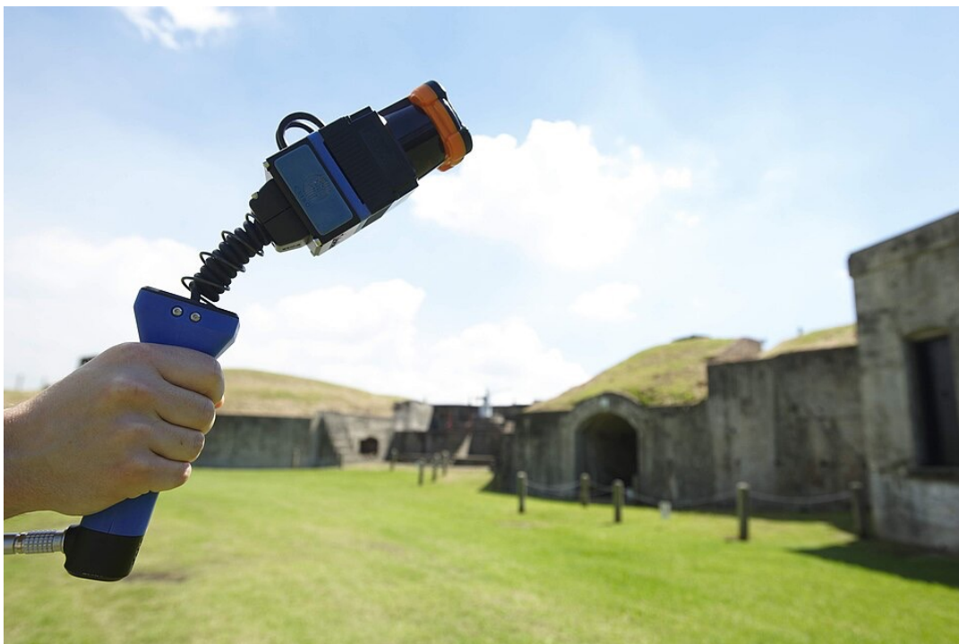
Figure 5: Handheld LiDAR scanner and an industrial-grade MEMS inertial measurement unit (IMU) mounted on a simple spring mechanism
