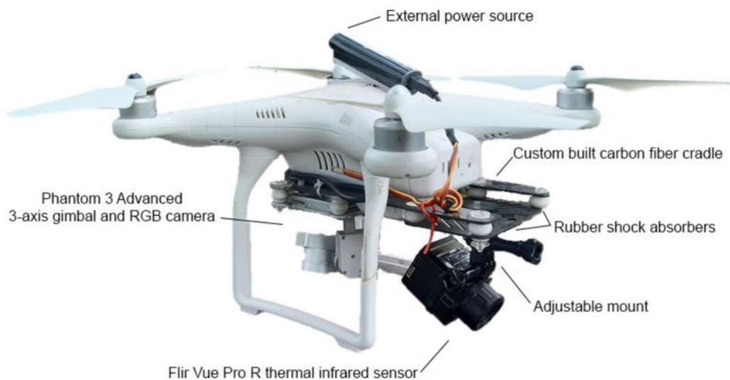
Figure 3: DJI Phantom 3 Advanced drone carrying a true-colour (RGB) camera and a Flir Vue Pro R (FVP) thermal infrared sensor fitted on custom cradle.
