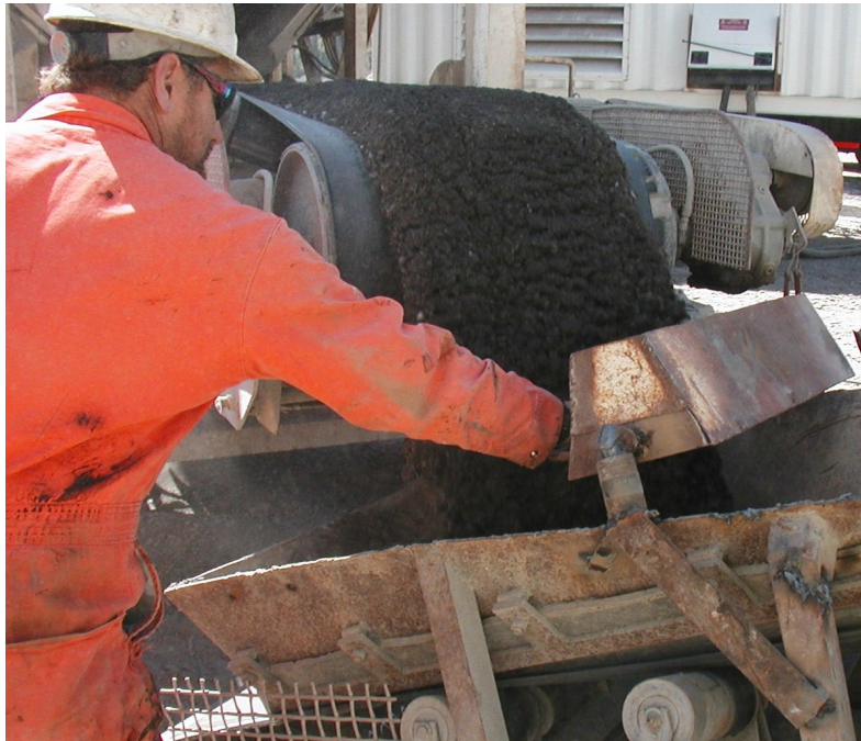
Figure 4: Sampling Device Cutting Across Flowing Stream.
