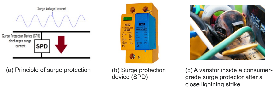
Figure 9: Surge Protection for electrical systems.
