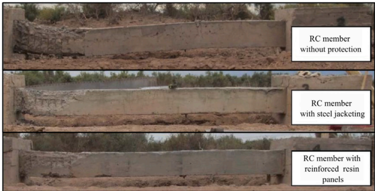
Fig. 31. Member retrofitting impact
