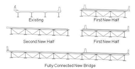
Figure 23 Sketches showing a half-width construction staging sequence
