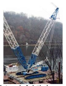
Figure 3 Photograph of a lattice boom crawler crane
