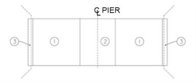
Figure 22 Sketch showing a sample deck placement sequence
