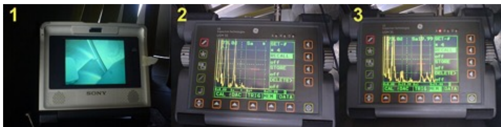
Figure 4: NDT, Ultrasonic Testing of an V2500 engine blade route
