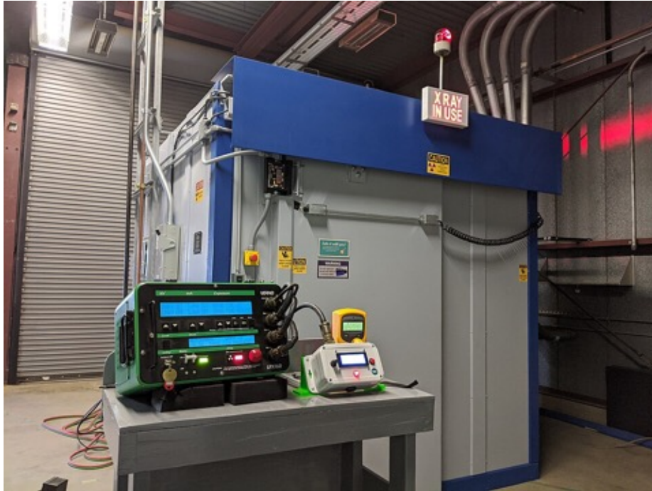
Figure 13: Non-destructive testing (NDT): X-ray vault used in radiography testing
