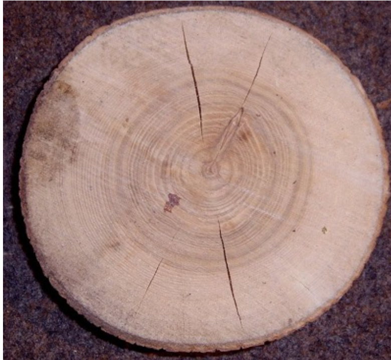
Figure 12: Cross-section of wood showing heart shakes
